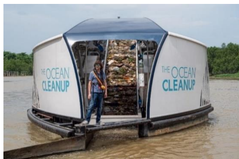
Figure 21 – The Interceptor, made by the company Ocean Cleanup, adapted to clean up plastics in rivers (The Ocean Cleanup, 2019).
